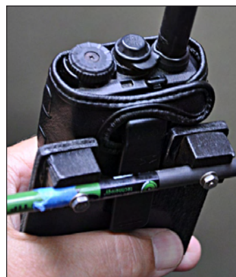
The HT mount is hardboard and some wood scraps.
