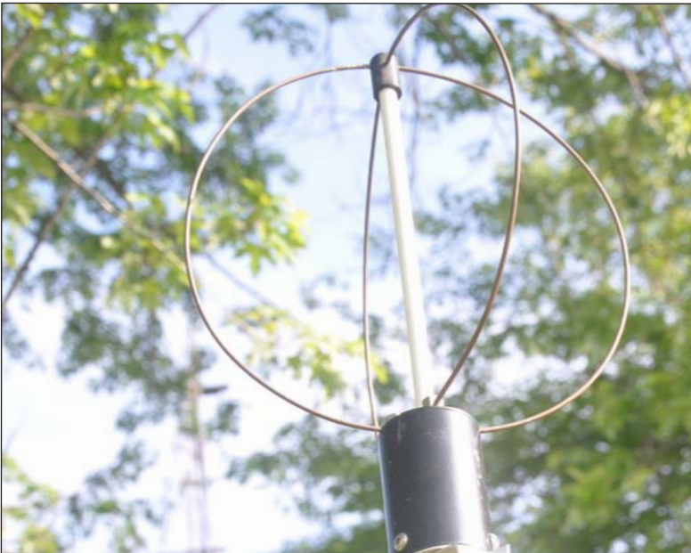
An "eggbeater" antenna to receive satellite UHF transmissions.
