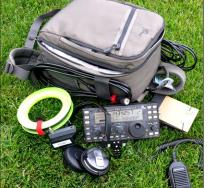
50' lengths of antenna wire, adapters, and a couple of 1-oz weights to get one wire into a tree; paper log and dupe sheets; soft carrying case.
