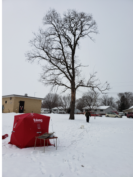
Drew operated from his ice shanty using a 40' end feed wire
